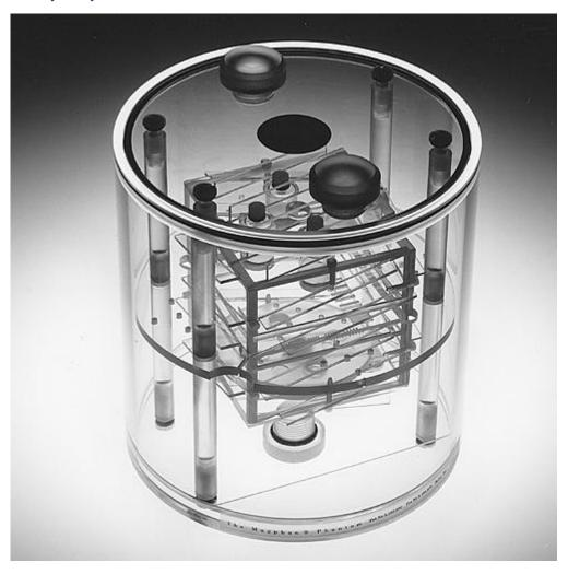
**Test Cube:** Both the cylindrical and spherical Magphan® use a 10cm test cube for image quality measurements. Manufactured from 6mm-thick polycarbonate plastic the test cube has an outer diameter of 10cm. The test cube contains the slice thickness ramps, sensitometry vials, a high resolution test plate and a low contrast disk.
